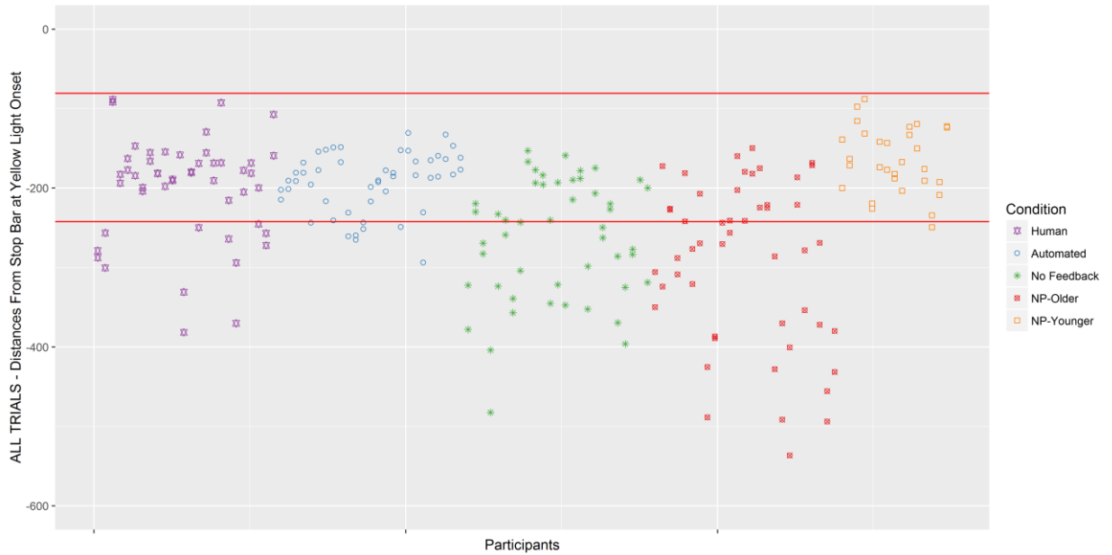
Figure 4.1 Scatterplot of distances from the stop bar at yellow light onset. Zero on the y-axis represents the stop bar, and the horizontal lines outline the dilemma zone. Points plotted at the same x value are from the same participant.
